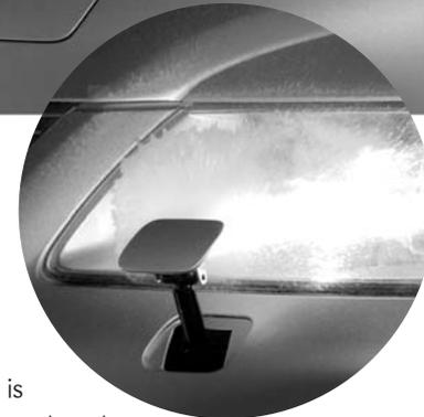
A special system takes care of cleaning the headlights, which is effective at any speed and does not dim the light from the headlights while it is in operation. The system consists of extendable cleaning nozzles and high-pressure cleaning jets that do the cleaning and rinsing.
